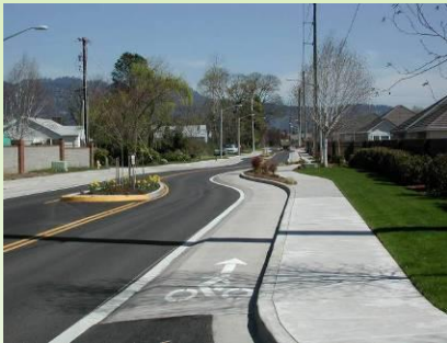
Figure 6.11 – Example of a Raised Bicycle Lane on Ayres Road in Eugene, Oregon
