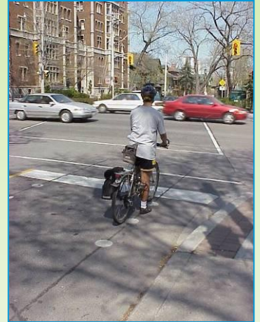
Figure 6.29 – “Three dots” Traffic Signal Actuation Indicator
