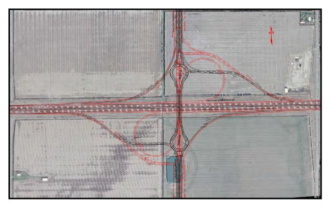
The proposed Highway 401 Interchange will be located approximately mid-way between the adjacent underpasses: 9<sup>th</sup> Concession Road and 10th Concession Road / County Road 17. As the new ramps associated with the Lauzon Parkway Interchange will extend beyond 9<sup>th</sup> Concession Road and 10th Concession Road / County Road 17, the potential impact to these existing bridges was reviewed.
